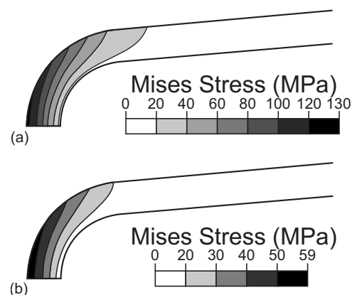
Fig. 15 Mises stress contours when the heat pipe is functioning: (a) Mises stresses for Mach 6 with nickel-based superalloy Inconel 625; and (b) Mises stresses for Mach 8 with niobium alloy Cb-752
