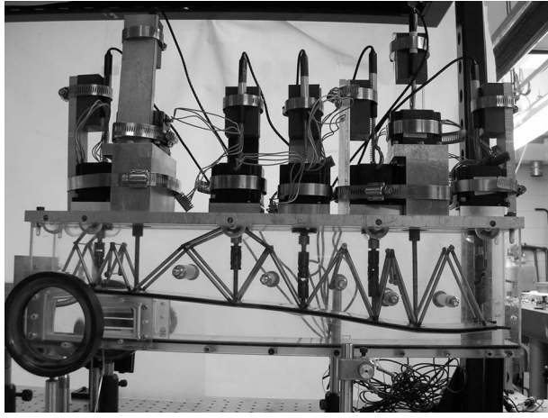
Fig. 1 A photograph of the morphing nozzle as installed in the in-draft wind tunnel. Visible are the curved morphing surface, the actuators, and the linear potentiometers used to control the system position.
